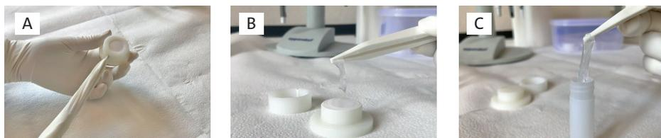
Image 12. (A) DGT opening; (B) Chelex-100 peel off; (C) Chelex-100 being placed in a sample tube (Source: UNICA).
