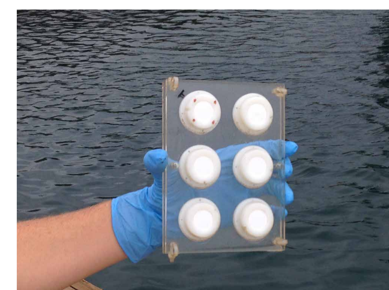
Figure 2. DGT assemblage after the exposure (Source: ITC)
