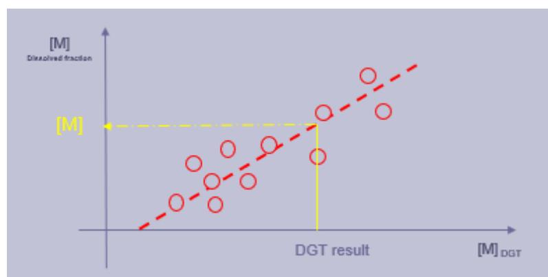
**Figure 7:** Illustration of the relationship  $[M]$  in the dissolved fraction and in DGT,
