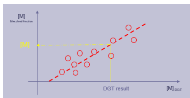
Figure 2: Illustration of the relationship [M] in the dissolved fraction and in DGT, [M]_{\text{Dissolved fraction}} = \text{slope} \times [M]_{DGT} + \text{intercept}
