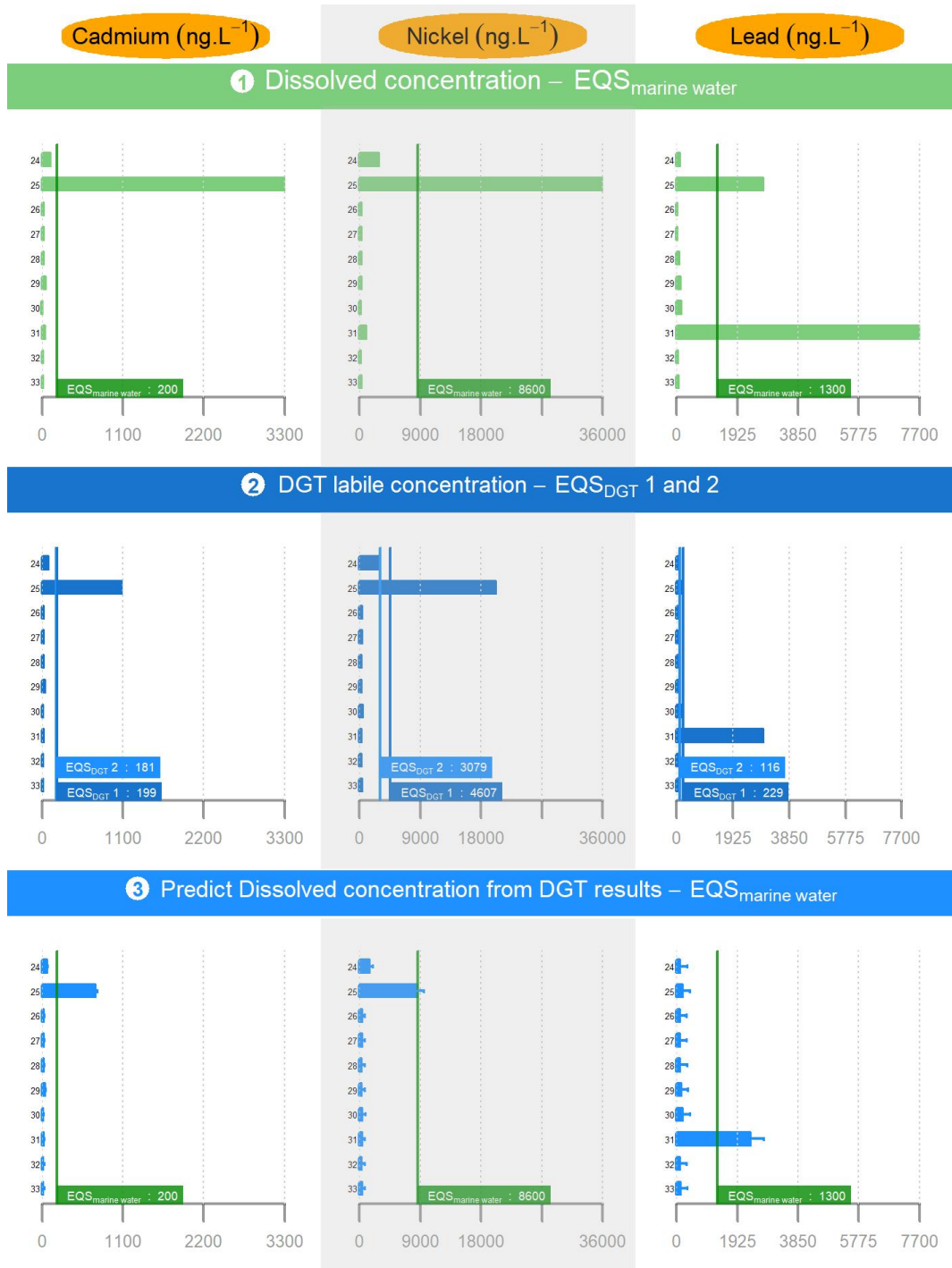
Figure 3: Comparison to EQS per sites sampled in 2022 within additional sampling campaign (MONITOOL extension) for cadmium, nickel and lead: 1 Measured dissolved concentration (in green) and indication of EQS marine water ; 2 Labile DGT concentration (ng.L -1 ) (in blue) and indication of (A)-EQS DGT n°1 & 2; 3 Predict dissolved concentration from DGT results (Eq. 2) and indication of EQS marine water .
