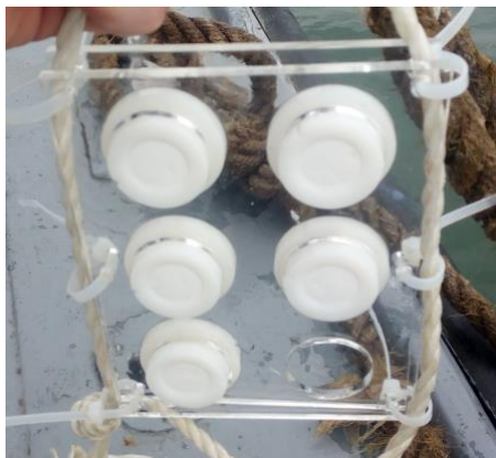
Figure 2 DGT devices mounted in plexiglass frame for deployment in Dublin and Cork.
